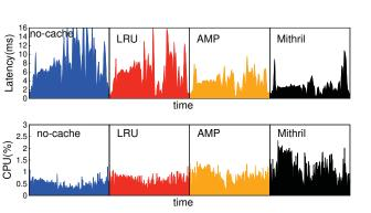
Figure 8: Latency and CPU usage of using no cache, LRU, Amp and Mithril-LRU. On the top, each latency point is the average latency of 40000 requests. At the bottom, it shows the relatively increased CPU usage of Mithril due to mining and prefetching, compared to LRU and Amp, the increase is less than 1%.
