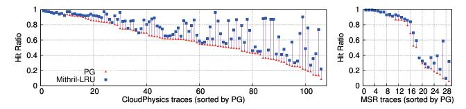
Figure 3: Hit ratio of PG and Mithril for 106 CP traces and 29 MSR traces sorted by PG hit ratio. Hit ratio of LRU omitted as it is similar to PG (Pearson r = 0.995 compared to r = 0.742 for LRU and Mithril). Compared to PG, Mithril overall provides significant improvement, even though parameters are not fine-tuned for each trace.
