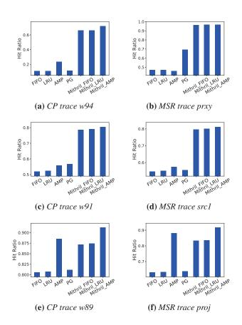
Figure 5: *Hit ratio of different algorithms. Example traces where* Mithril *significantly improves hit rate (top two), where* Mithril *shows modest improvement (middle two), and where* Mithril *shows little or no performance gain (bottom two).*
