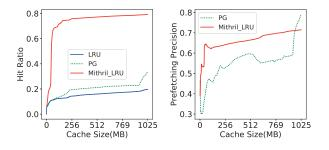
Figure 6: *Hit ratio curve and prefetching precision of* LRU, PG and Mithril Left: Mithril outperforms LRU and PG. Right: The prefetching precision of Mithril is higher than PG and both two curves are not monotonic.
